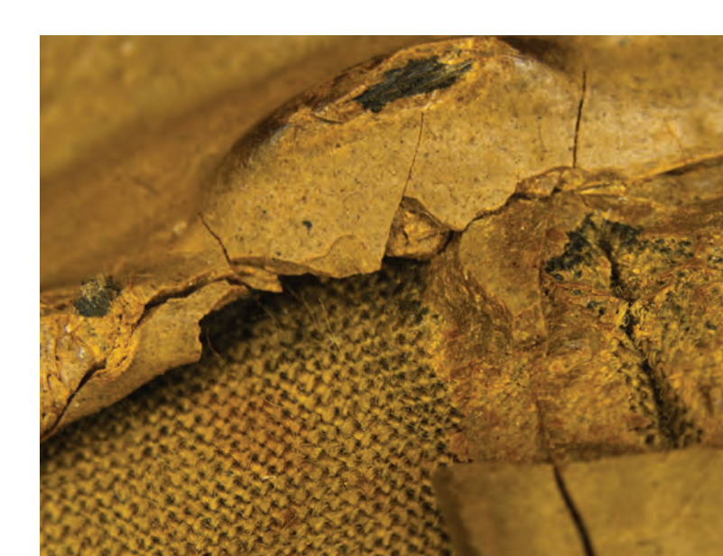
Gas mask ST-38, cracked rubber coating materials (mag. 10x). Photo: Indra Saulesleja
