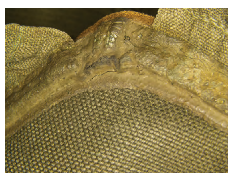
German S-maske, cracked rubber coating materials (mag. 10x). Photo: Indra Saulesleja
