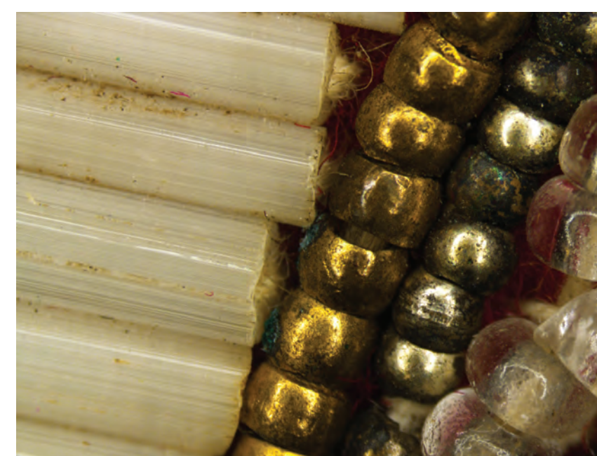
The development process of corrosion products between glass straws and bronze beads (mag.35x). Photo: Indra Saulesleja
