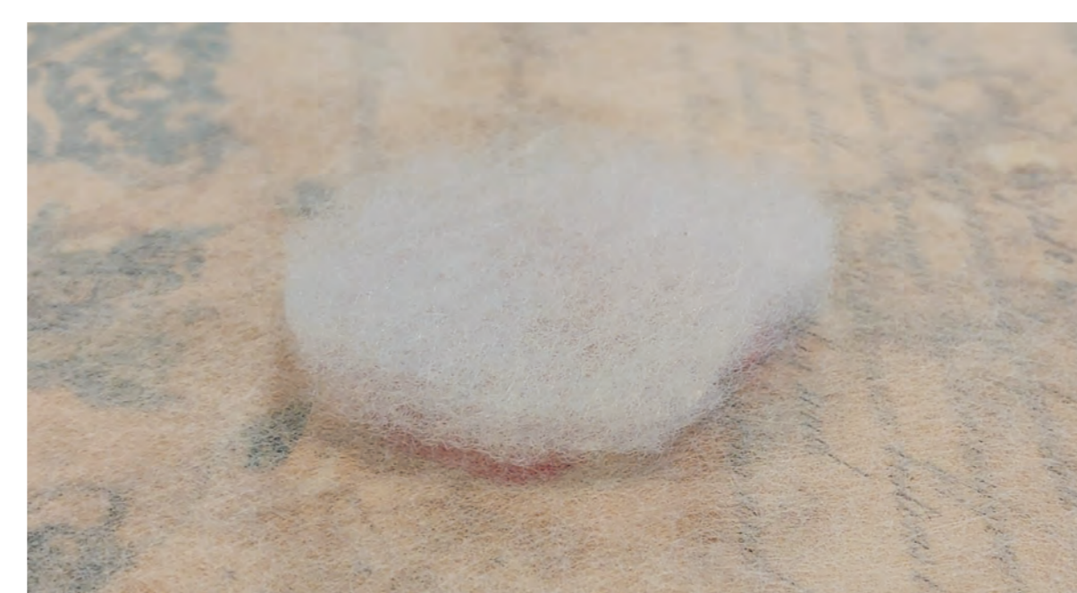
(Fig. 9) GV 426 Sintepon padding for the lacquer seal
