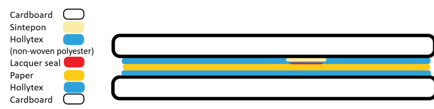
(Fig. 8) GV 426 Drying by pressing between layers of cardboard, non-woven polyester and the padding of the lacquer seal
