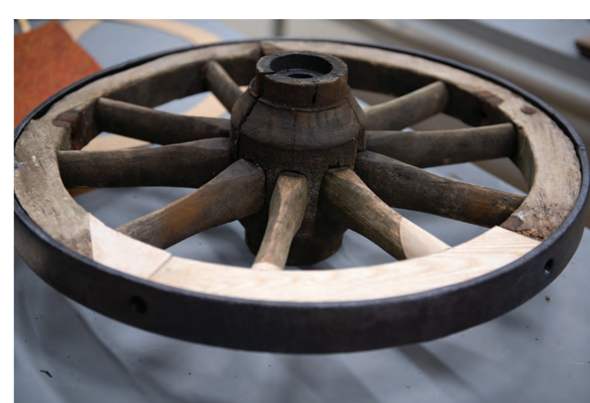
7. Front wheel during restoration
