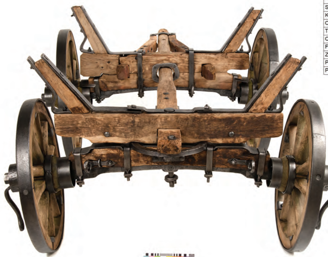
2. Wagon (front axle) after restoration
