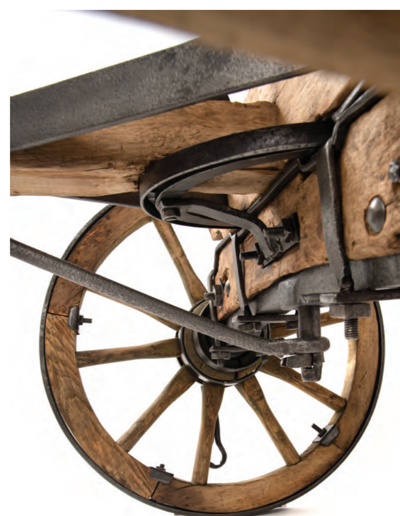
9. Front axle assembly after restoration
