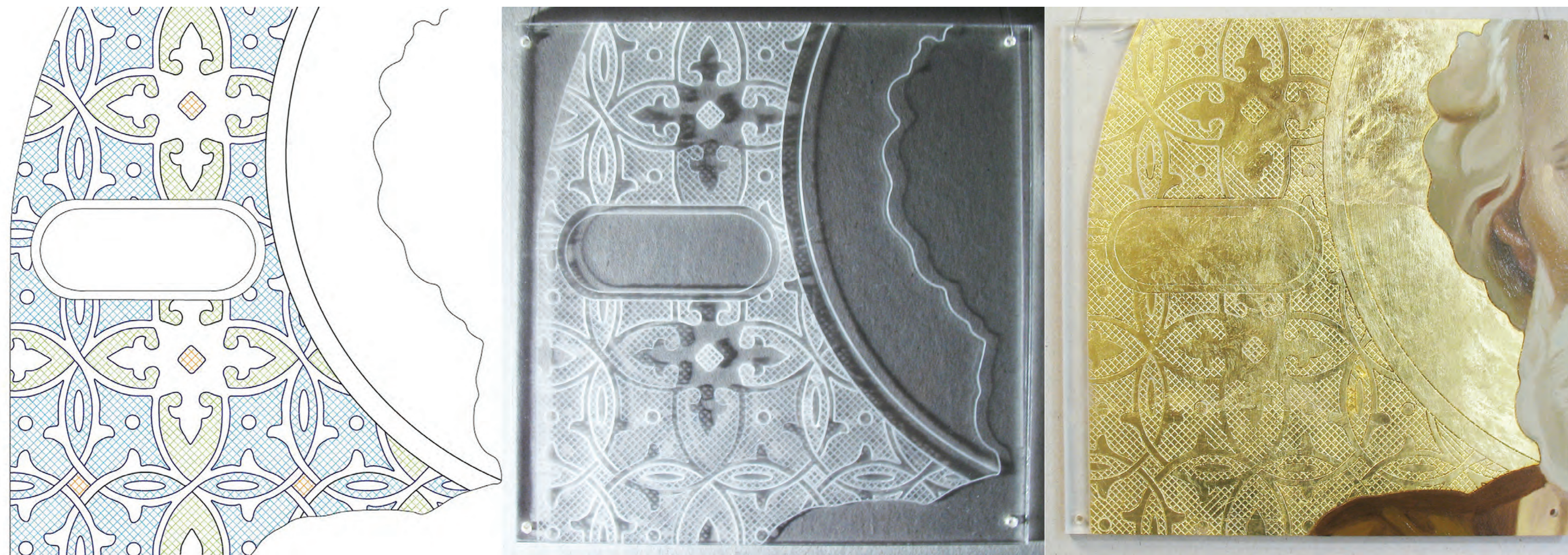
Fig. 2. Preparation of an example – the pattern was developed using Adobe Illustrator, and engraved in the organic glass sheet with a laser, then gilded and painted
