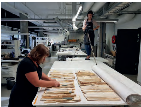
Image 2. Mass treatment method for relaxing and flattening by using a Gore-Tex sandwich (local government records from 1860–1918)
