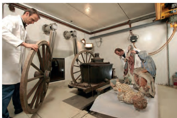
Image 2. Setting ethnological artefacts and wooden polychromed sculptures inside the irradiation chamber before their irradiation for insect eradication
