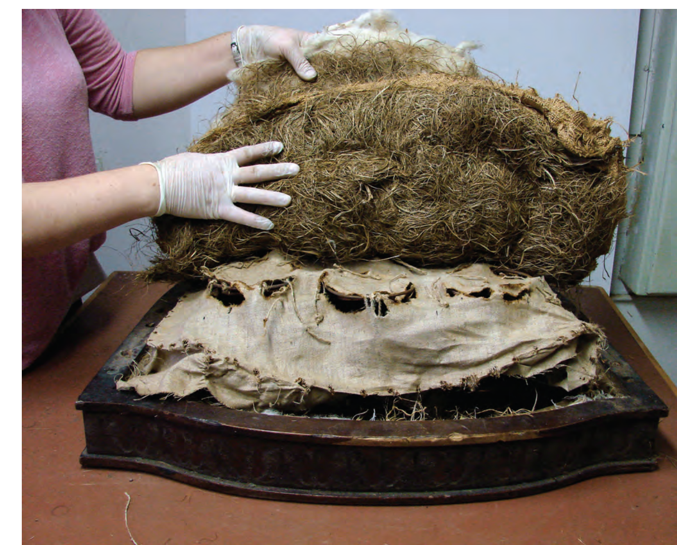
Process of restoration: The upholstery of the seat is worn out, in a few places the springs are covered in corrosion products, thus damaging other upholstery materials. Damage upholstery removed from the seat.
