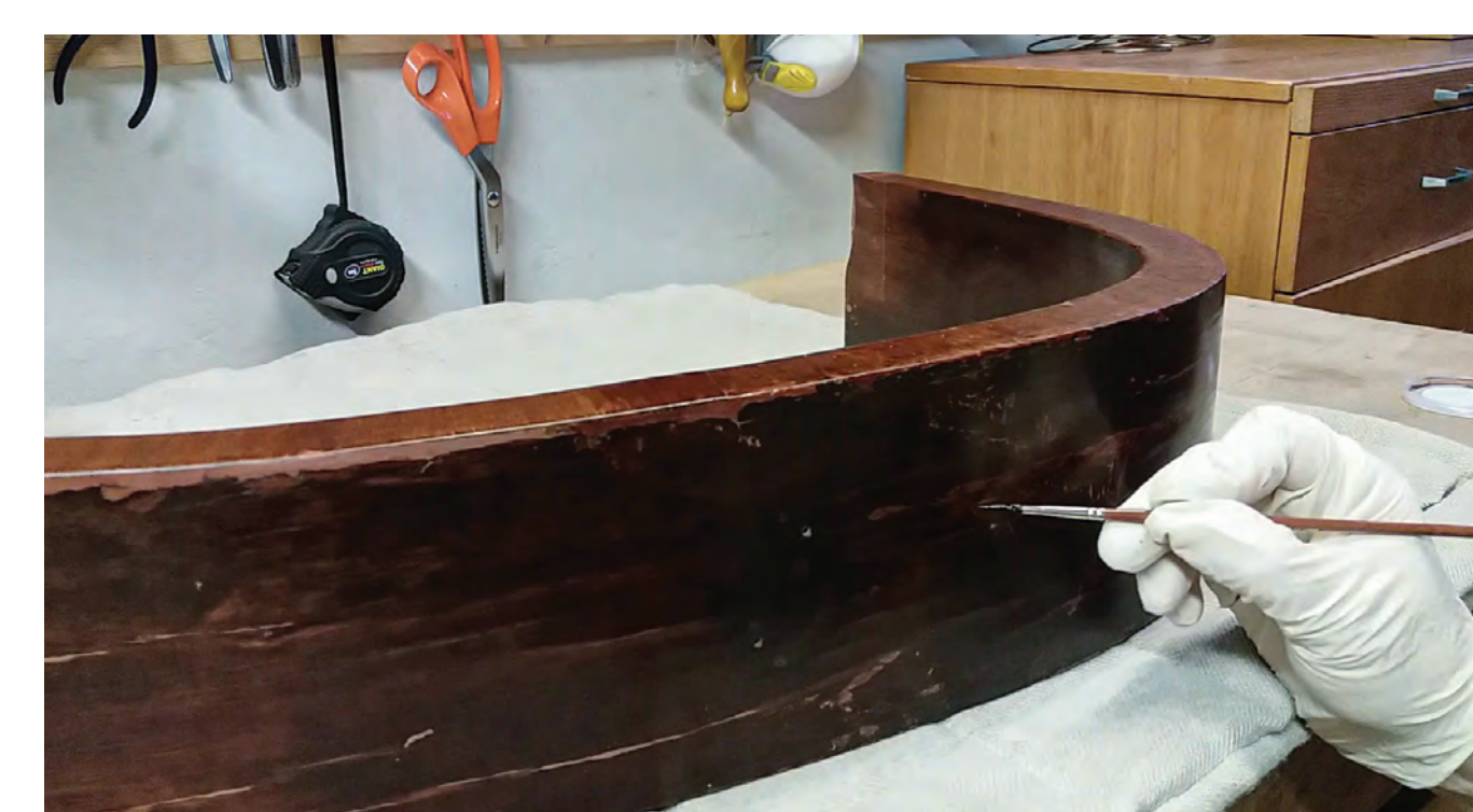
Process of restoration: the areas filled with filling paste are then varnished and toned with ethanol-based woodstain.
