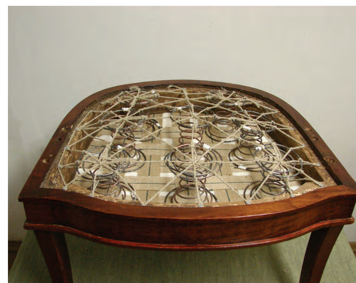
Process of restoration: new upholstery is created by using the same materials as the original.
