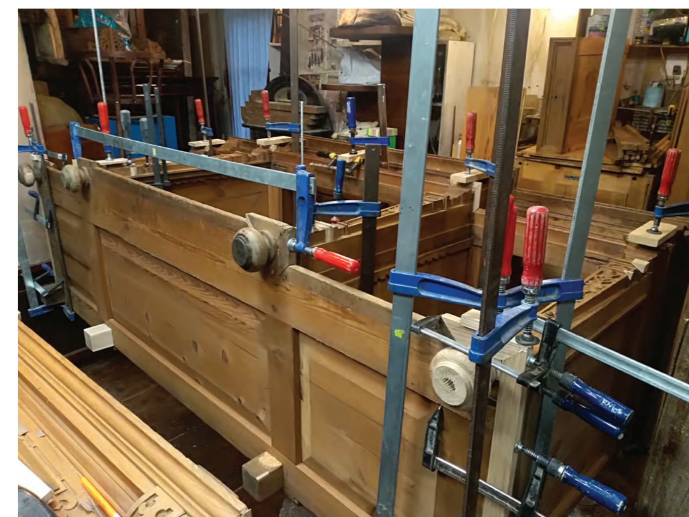
Fig. 7. The process of gluing the structure of the sideboard. Photo: Aigars Pilenieks
