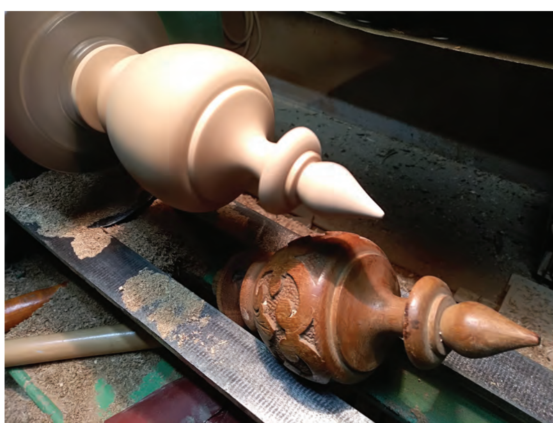
Fig. 9. The process of making the missing turned part. Photo: Aigars Pilenieks
