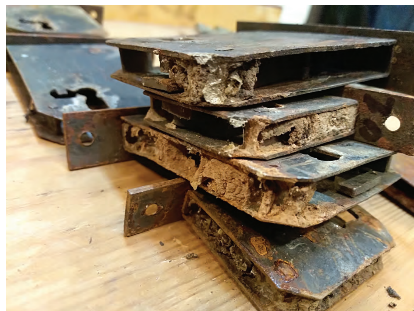
Fig. 6. Damaged sideboard locks before restoration. Photo: Aigars Pilenieks
